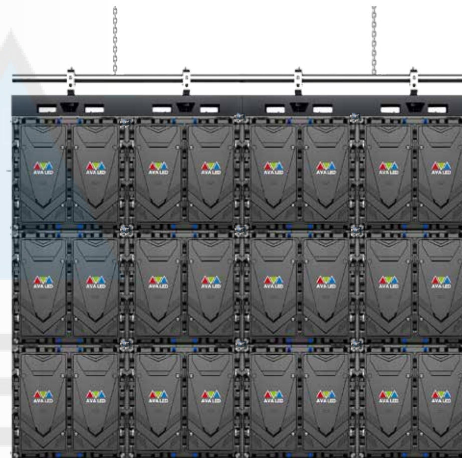
Picture 10-2. Hanging installation
